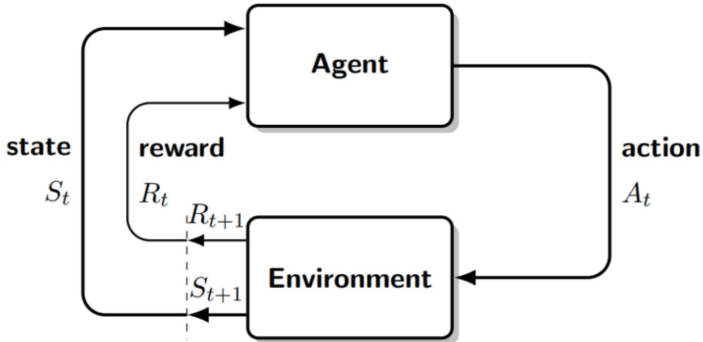
Figure: The agent-environment interaction. Adapted from Sutton and Barto (2018).
